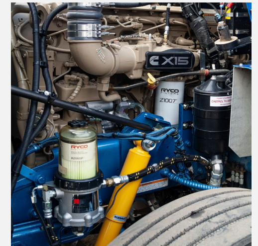
Ryco fuel filtration for Cummins X15 Diesel Engine
