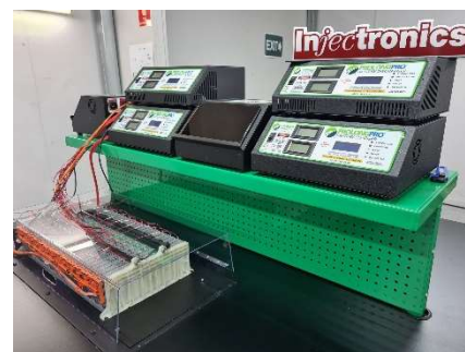
Hybrid EV battery testing station
